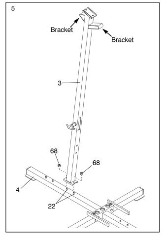
Slide the Butterfly Upright (2) onto the indicated 5/16" x 2 1/2" Carriage Bolts (22) in the Butterfly Base (8). Hand tighten a 5/16" Nylon Locknut (68) onto each Carriage Bolt.
